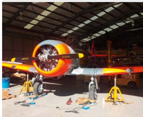
Harvard XSA in for an engine change.
