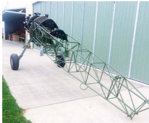
Stearman STM refurbishment.
