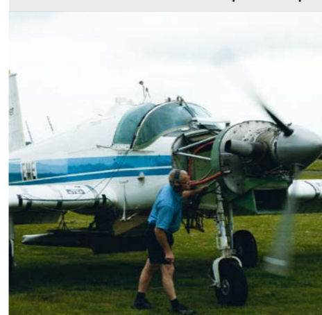
Paul Waterhouse checking a recently maintained PT6.
